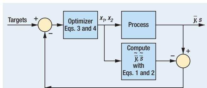
FIG. 3 CMPC system for the 2x2 example.
